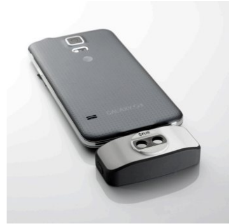
Figure 25.3 2015: FLIR One, an accessory to iPhone and Android mobile phones. Weight: 90 g (3.2 oz.).
